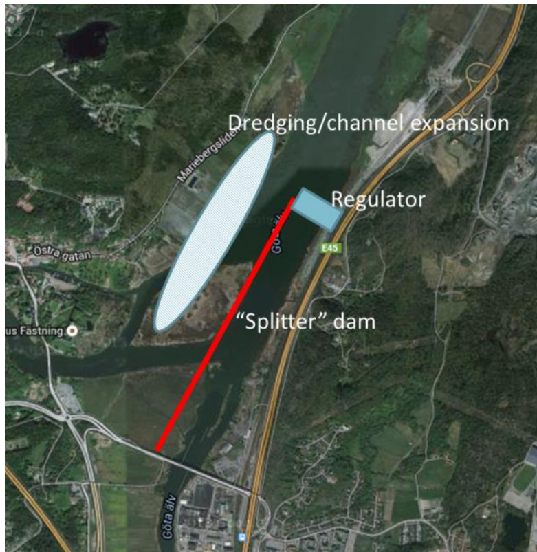
Figure 2 Barrier in the upstream section of the Göta älv
