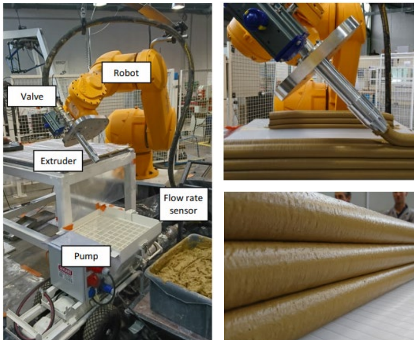
Figure 13 View of the 3D printer used by the University of Bretagne (Perrot et al., 2018).
