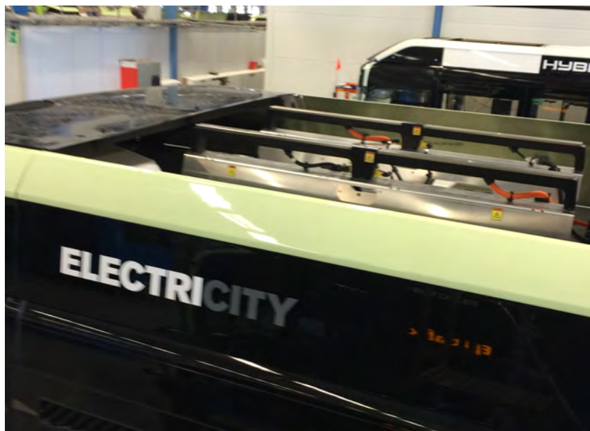
Figure 3.1 Top of the bus, the rails that the pantograph connects to during high power charging are shown.
