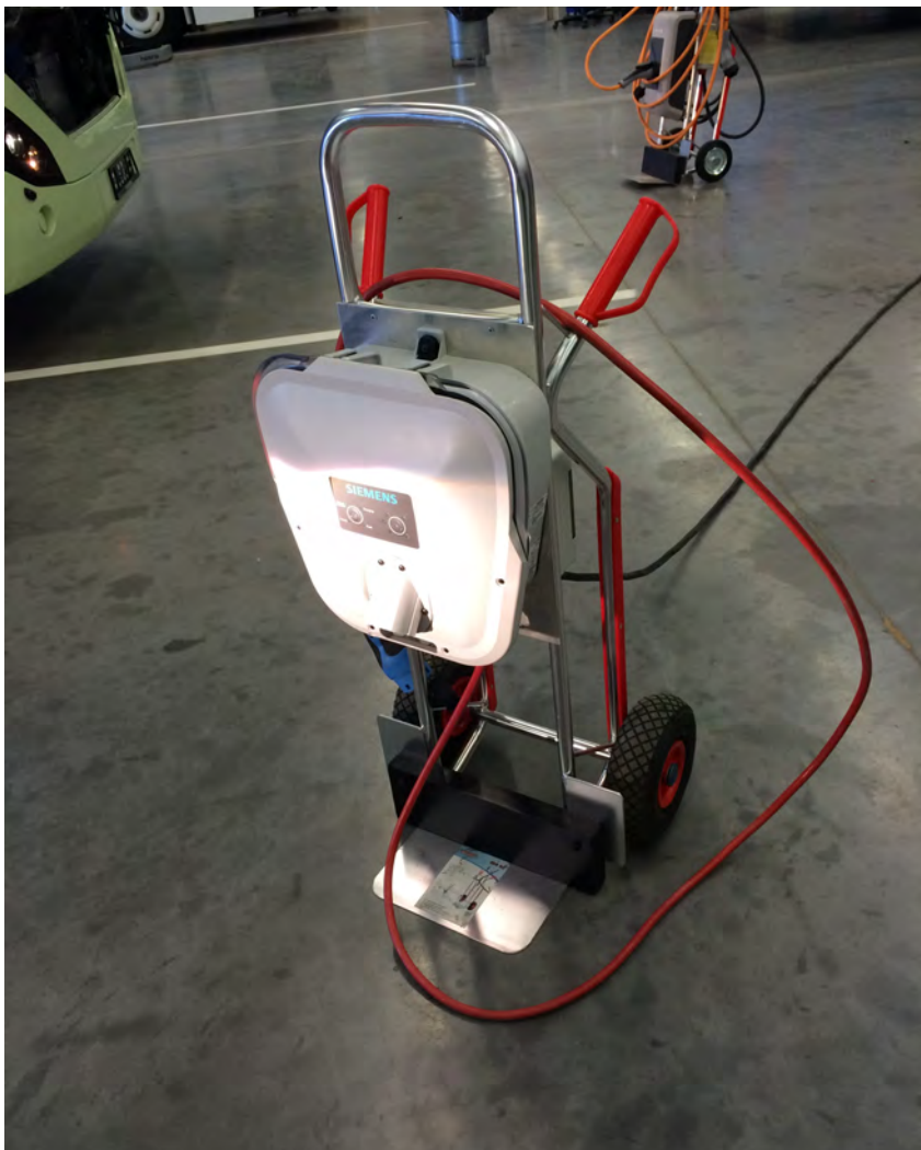
Figure 3.3. Charge box used for low power charging.
