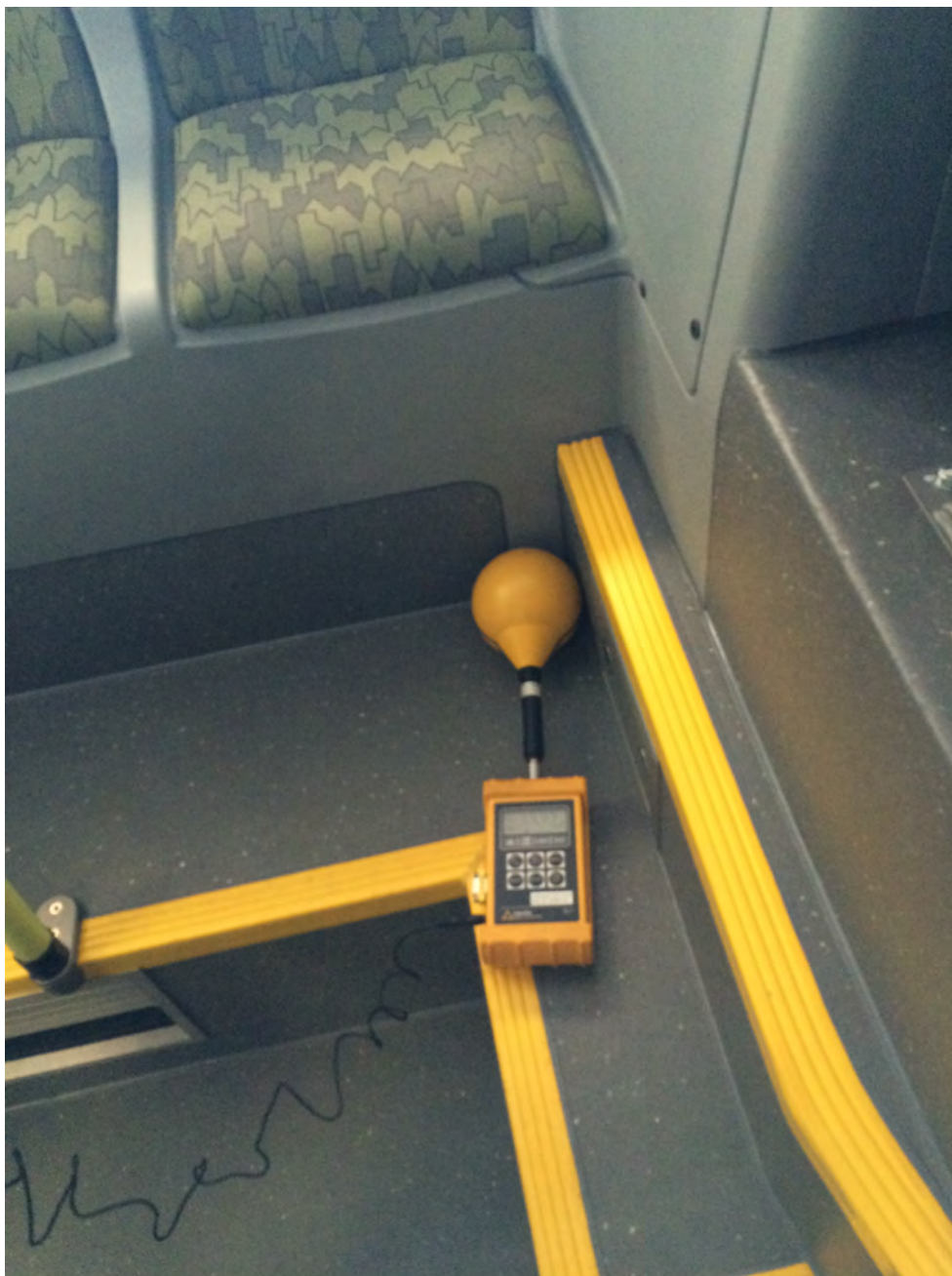
Figure 2.2. Measurement point: the middle seat of the back, at the floor.
